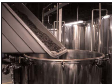
Vanilla beans are put into stainless steel extractors to produce America's favorite flavor... vanilla.
